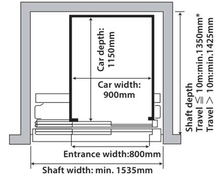
\* Min. 1400mm when Double Isolation Unit for Absorbing Vibration and Sound is applied.
